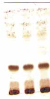
After spraying with 10% Eth. H 2 SO 4
