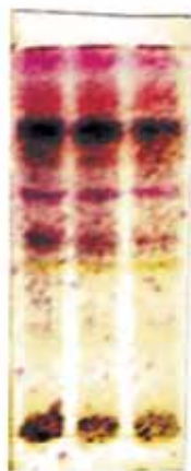
After spraying with VSA and heating at 110°C
