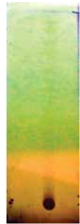
Iodine Vapour TLC Banafshah - Chloroform extract
