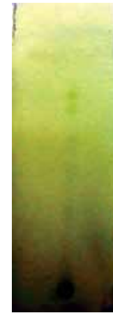
Iodine Vapour TLC Banafshah - Chloroform extract
